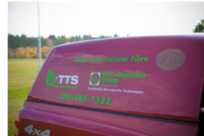
Tekle Technical Services, Drayton Valley, AB Truck cabin made of wood residues
