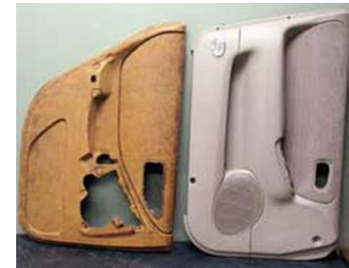
Car door panels made from fibre mats
